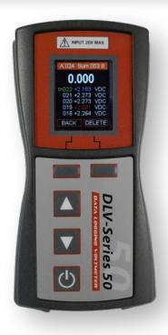
The DLV50 data logging voltmeter automatically measures and records cell voltages in less than 1 second and then increments the cell counter. This enables the user to take hundreds of cell voltage readings from a string of cells without being interrupted to write down a reading or even push a button.
